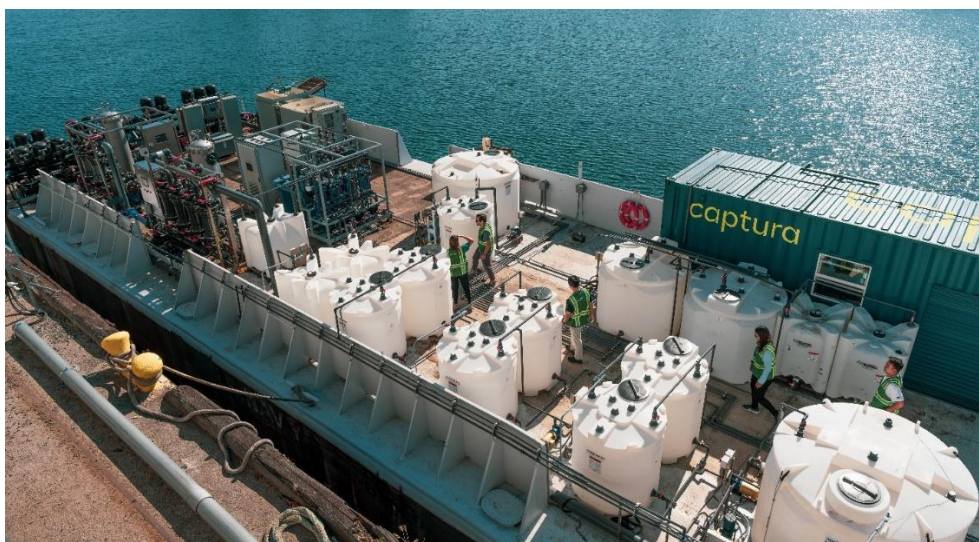
Figure 1. Captura's operational DOC pilot system at AltaSea at the Port of Los Angeles
